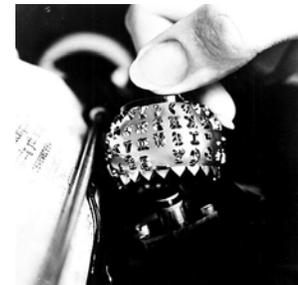
Introduced in 1961, the IBM Selectric was an amazing electronic mechanism. It ingeniously used a machined, steel globe or golf-ball type-element populated and engraved with raised letters of every character in the alphabet. The ball could be easily changed to permit typing in different fonts and languages. I found it amazing to watch
