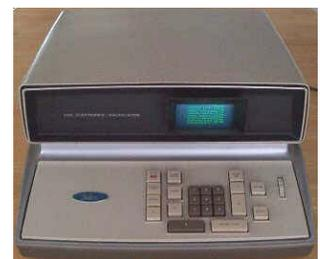
The EC-130 is generally regarded as the first transistorized electronic calculator.
